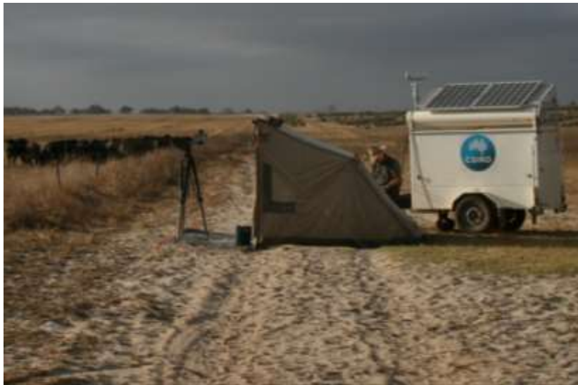
Figure 3. Open path lasers have been used by CSIRO on Avoca to measure methane emissions form cattle grazing perennial shrubs.
